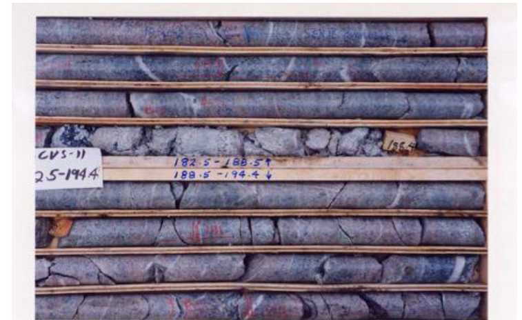
Quartz stockwork zone with bornite-chalcocite-quartz veins. Note sericite II overprint on pink K-spar alteration, which displays specks of martitized magnetite altered to hematite.
